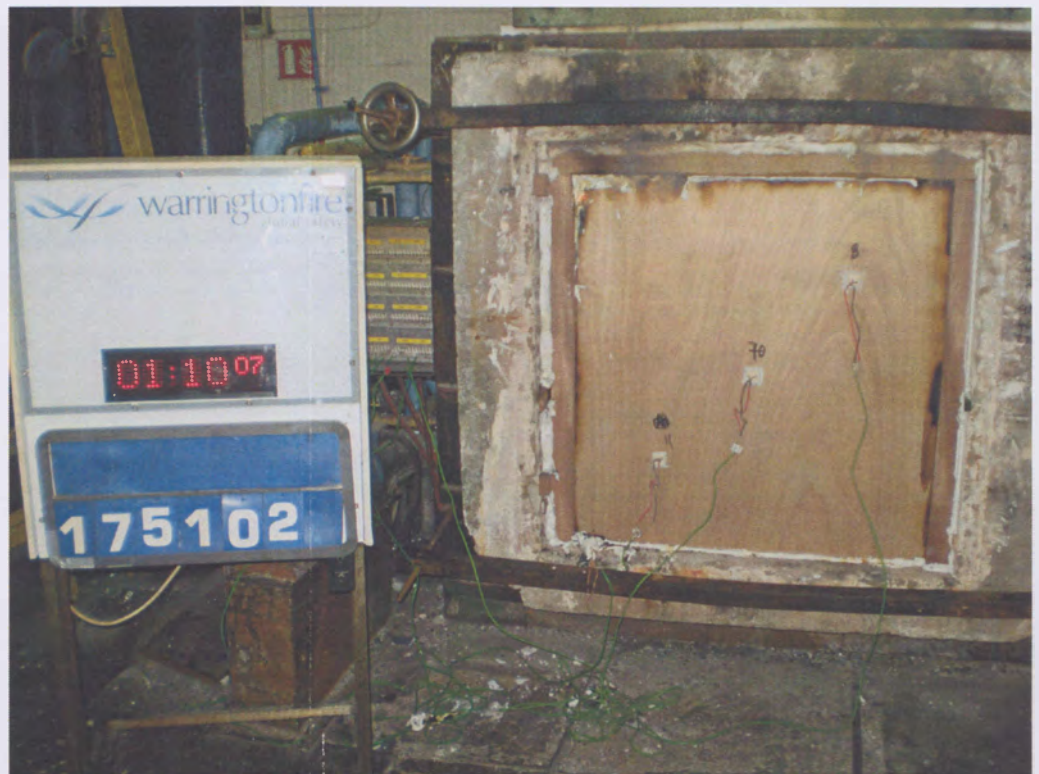
The unexposed face of the doorset after a test duration of 70 minutes
