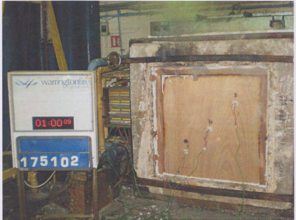
The unexposed face of the doorset after a test duration of 60 minutes
